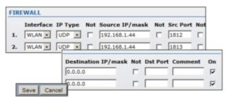
Firewall entries can be specified by using the following criteria:
