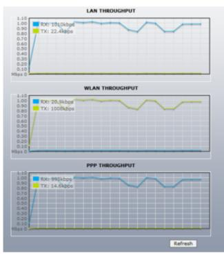
**Show Throughput:** selection opens statistics window which continuously represents the current data traffic on the LAN, WLAN and PPP interfaces in both graphical and numerical form. The chart scale and throughput dimension (Bps, Kbps, Mbps) changes dynamically according to the mean throughput value.
